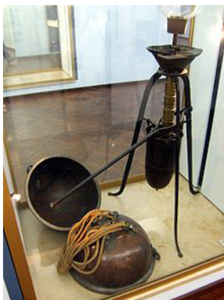
The original Magdeburg hemispheres and Von Guericke's vacuum pump in the Deutsches Museum, Munich, Germany
