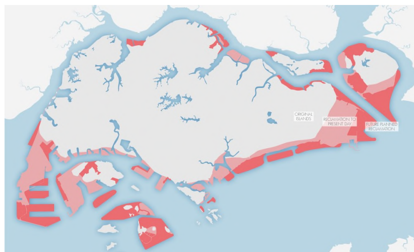
- Singapore Expansion - Pink areas illustrate the land created up to 2013. Red areas illustrate planned future expansion.
