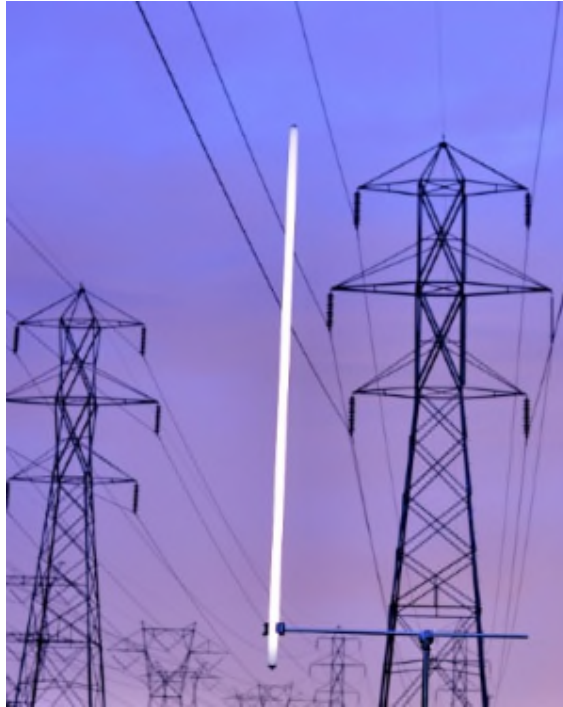
A fluorescent tube lights up when placed under high power transmission lines.
