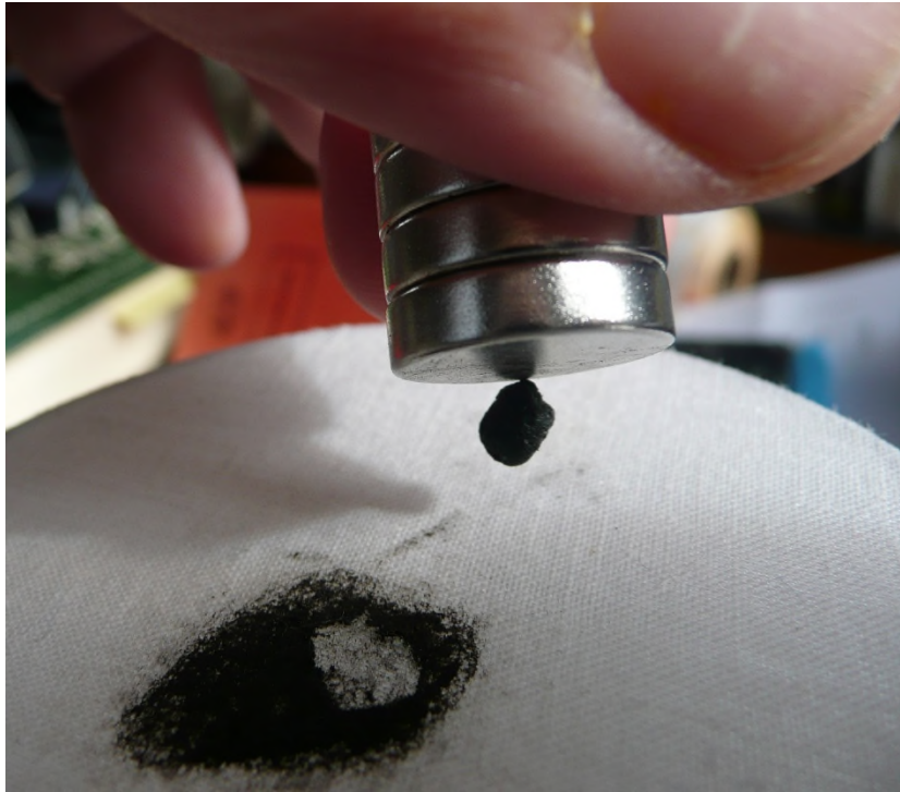
ABOVE: The black lump adheres magnetically to a set of 8 neodymium round magnets (each 15mm x 4mm)
