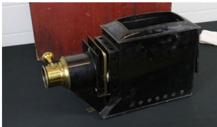
19 th century Magic Lantern Projector, made of tinfoil and brass. The source of illumination was inserted into the black box.
